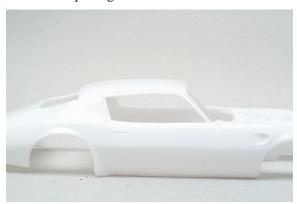
The kit has no drip-rail trim (optional on the real cars), which makes the fix a matter of sanding the openings to match a photo of a 1/1 Firebird. I reshaped the window with a 320-grit sanding stick and finished with 600-grit sandpaper. Additionally, I scribed around the fender vents because they are separate units on the real cars. I inserted a metal pin into the sideview mirrors for a stronger attachment and drilled a mounting hole for them in the doors.
