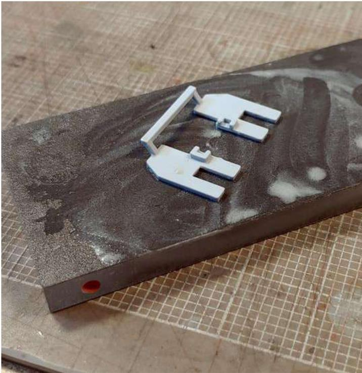
pads and sticks. Similarly, I find a tool like these much more controllable than a metal file, and given that they are wider, they are more conducive to finishing longer edges than a file or sanding stick. All of this is holding the work (Model or Part) stationary and moving the tool (Super Sanding Block). These blocks also impressed me in the converse situation.
