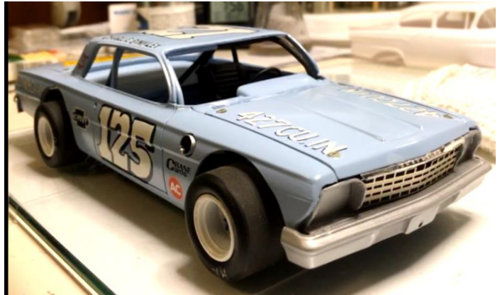
1962 Chevy Biscayne— resin body from MCW; built on a 1962 Pontiac Catalina chassis. http://www.mcwautomotivefinishes.com/resin/newstuff.html
