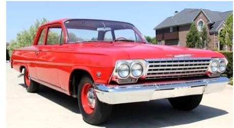
1962 Chevy Biscayne— resin body from MCW; built on a 1962 Pontiac Catalina chassis. http://www.mcwautomotivefinishes.com/resin/newstuff.html
